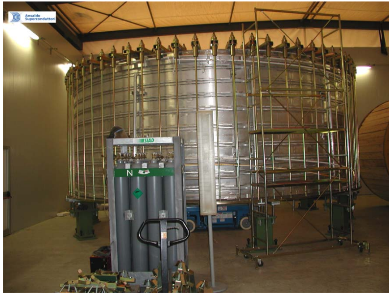
Fig. 7. CB-2 ready for impregnation at Ansaldo (Genova, Italy)
