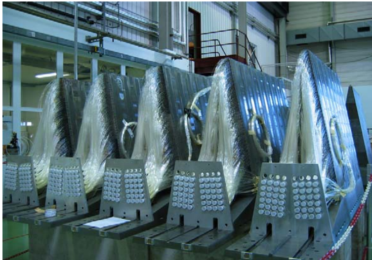
Fig. 15. HF wedges complete with quartz fibres inserted
