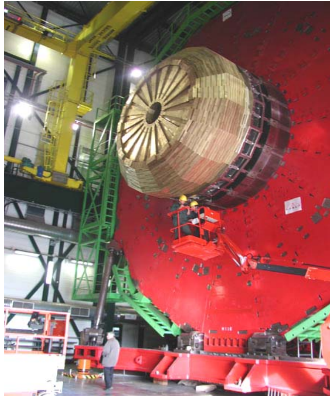
Fig. 14. HE-1 mounted on the first disk of the endcap yoke YE-1
