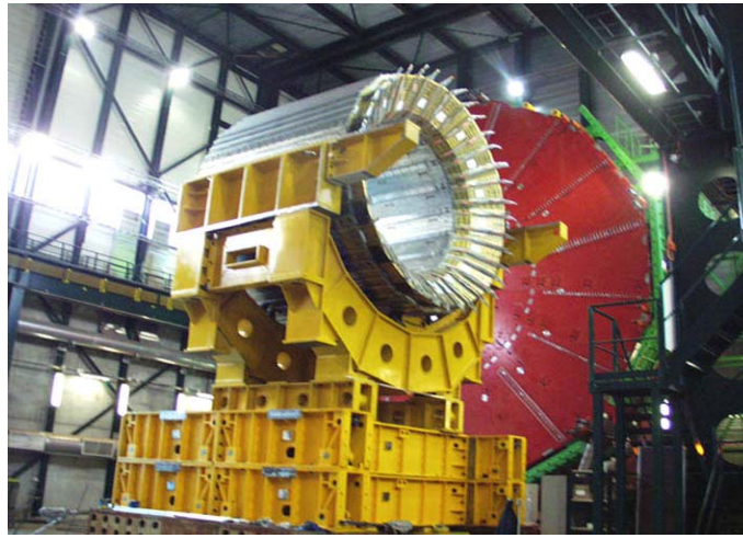
Fig. 13. View of the first half-barrel hadron calorimeter (HB+1) assembled in SX5 and sitting in its cradle. The cradle is used for the assembly and for the insertion into the coil
